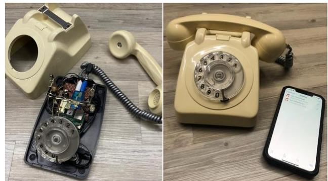
**Figure 2: The left side shows the interior of our prototype with Raspberry Pi 3 and USB audio adapter. The right side shows the retro-inspired audio guestbook prototype with wireless hotspot for easy access to recorded messages folder via one smartphone app.**
