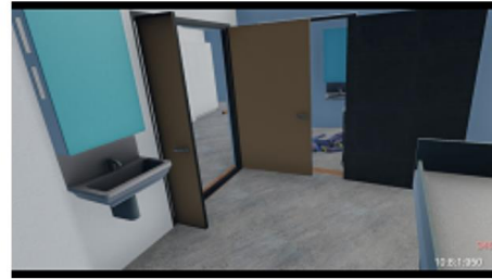
(b) The double-door entrance as seen from inside of the patient room. Here the double-door is open and is seen obstructing the entrance to the bathroom for people and artefacts to pass through.
