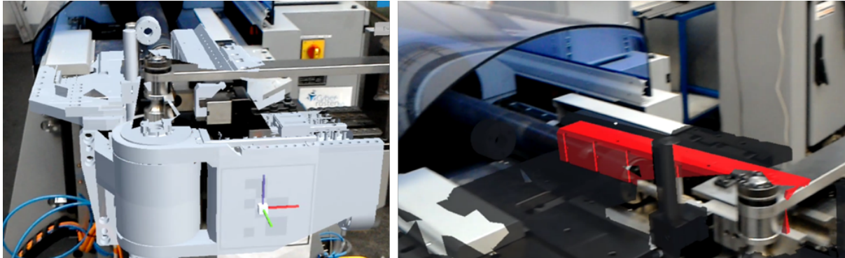
Figure 4: Contextualization of set-up instructions by marking the assembly sites on a bending machine – e.g. the green, blue and red axes on the left picture and the red area on the right picture.
