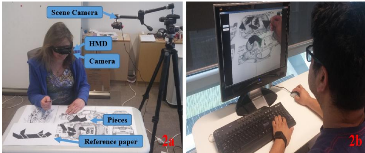
Figure 2: System setup for the mutual collaboration with the independent view. A local user wears an HMD to see the workspace and remote partner's annotations while assembling a model. A reference paper is placed at top right corner of the workspace, and another camera for remote partner's independent view is placed beside the local user (2a). A remote user watches the workspace with the independent view while drawing annotation with the mouse interaction (2b).
