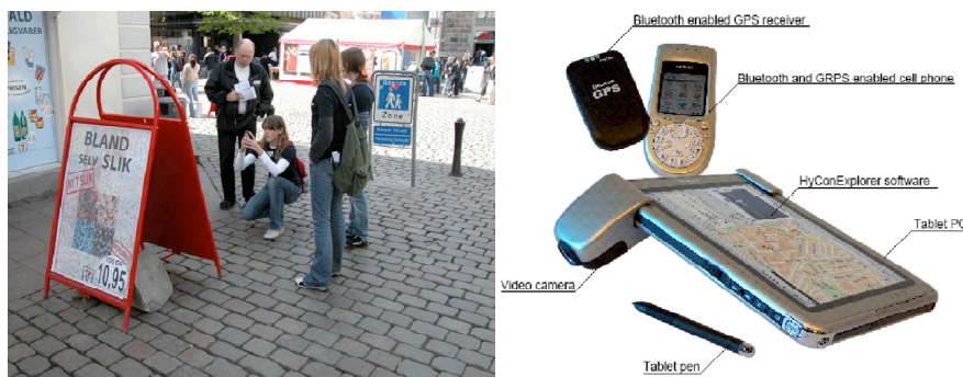
Figure 2 - The HyConExplorer prototype pack and the HyConExplorer in the field
