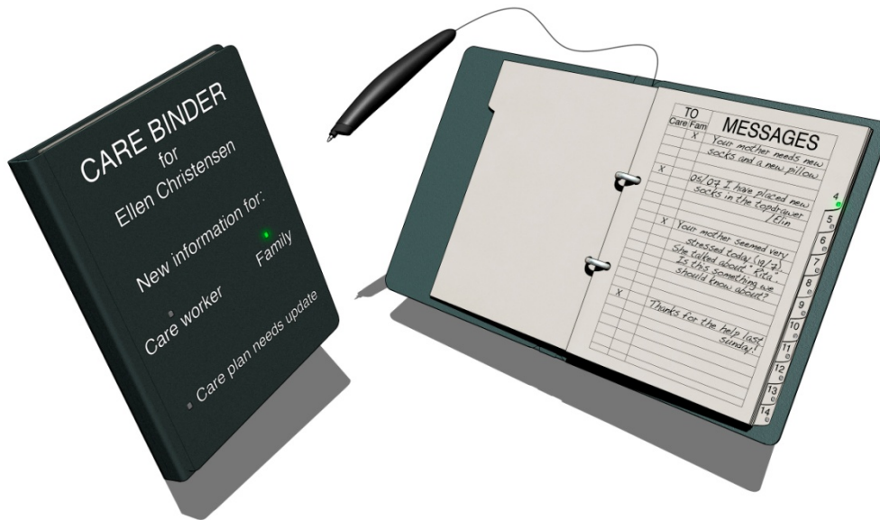
Figure 1. The augmented binder employs a pen for the digital capture of messages, and provide notifications of new messages employing RFID technology.
